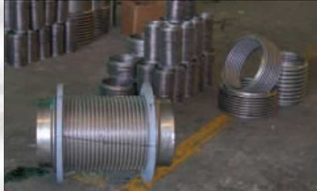
Single Exp. Joints in the Factory
